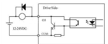
Figure 3.4: Output Interface Wiring
